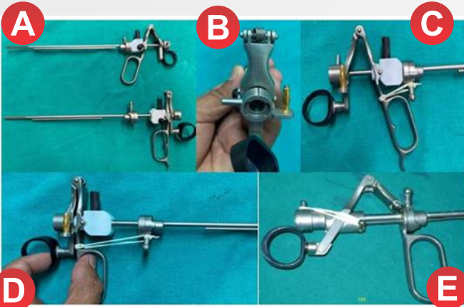
Figure: A – Normal working element and broken spring working element, B – Broken spring, C – Active working element tied with rubber loop at rest, D – Active working element with spring action, E – Passive working element
